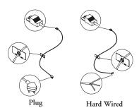
The Input Power Cable brings power from the building to the panel. It can be installed in the base opening of the panel to feed power up to the panel raceway or worksurface level. It can also be brought down from the ceiling to the workstation via a power plate.
