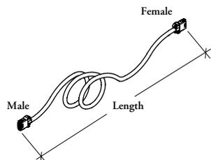
The Base Feed Extension Harness brings power from the Base Feed to the first Power Box included in the Power Kit – Library Table (THEPKL).
