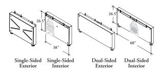
End Gables attach to the Truss (UMCT) to form the table chassis.
