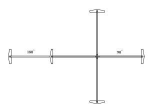
A Thin Panel span can be extended at 180° when a stabilizer foot is added where two Monolithic Thin Panels connect. A 180° span is limited to two Monolithic Thin Panels. When both panels are 66" high the span is limited to 72".
