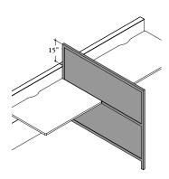
• For on-module applications where Lyft Thin Panels are higher than Leverage Panels, the difference can be no more than
