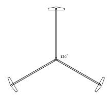
Monolithic Thin Panels can stand alone with two Stabilizer Feet or link to other Lyft Monolithic Thin Panels at 90° or 120° using one Stabilizer Foot per panel .
