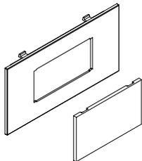
Communications Bezel converts unused openings in the Power/Communications Element to accommodate communication outlets.
