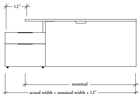
Extends 12" beyond the worksurface and the 12" extension is **not** calculated in the nominal dimension, the actual footprint will be 12" greater than the nominal width.
