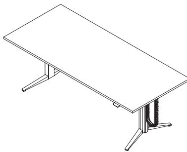
Vertical Wire Carrier (YEEE06) specified and installed on exterior of the frame's leg.
