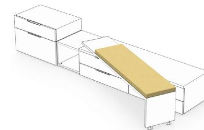
If 1.5 High storage is required with a 1 High Pivot Bench, there must be a 1 High storage unit between the two units to allow the bench to pivot
