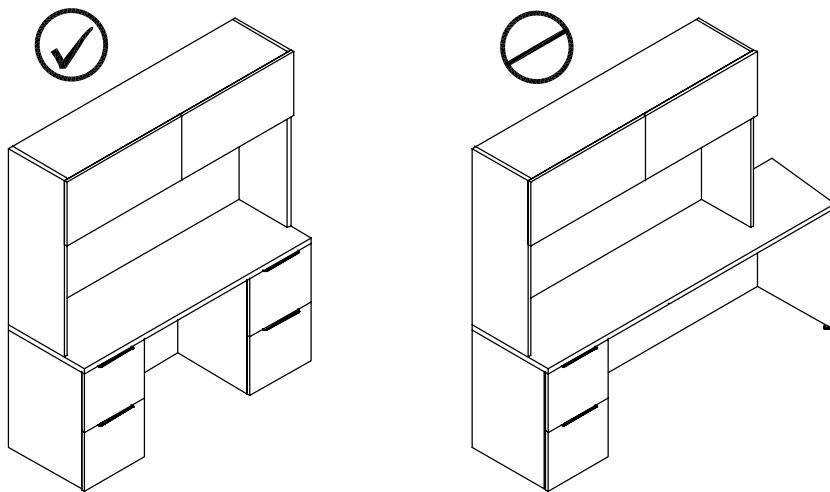
Both end gables of the hutch must sit over a storage unit to carry the load.
