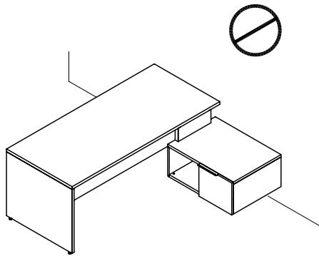
Run-Offs **cannot** connect to any wall-mounted storage units.
