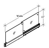
The Sliding Screen consists of two separate glass screens attached to a rail on rollers to provide user adjustable seated height privacy.
