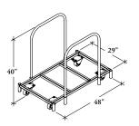
The Mobile Table Trolley is used for moving and storing tables and worksurfaces.
