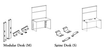
The Back Connection Kit is designed to connect a 2" Freestanding Screen to the back of a Modular Desk or a Spine Desk.
