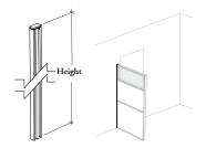
The Wall Connection Kit is designed to connect a 2" Freestanding Screen to a wall.
