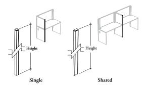
The Lateral Stabilizer – Elements is used to stabilize elements mounted on the side of a desk. It also acts as a finished covering.
