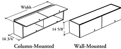
This cabinet is a metal mounted storage unit that provides above worksurface storage capabilities.
