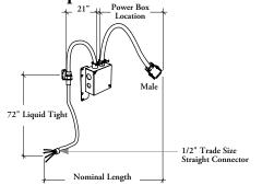
The NYC Split Base Feed connects to the building supply and routes power into the workstation from the wall or floor.
