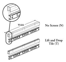
The Chicago EZ Fence Beam for Corridor is a key structural element of the product providing horizontal support for Floor or Modesty Screen – EZ Fence Beam-Mounted. It also carries electricity and data cabling across workstations.
