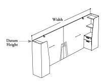
This screen with metal tower attaches to the side of a structural leg and provide space division and storage area to store garments and other items combined with optional filling or recycling/waste bins section.
