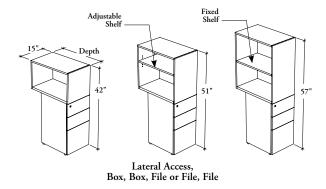
These beam towers provide different storage possibilities, while supporting the front of a worksurface and let a beam pass-through.
