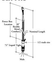
The Base Feed connects to the building supply and routes power into the workstation from the wall or floor.
