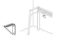
The Wall Anchored Stabilizer is used with a beam against a wall to maintain stability of the single-sided structure.
