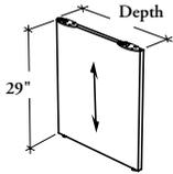
This support is an alternative to legs for Rectangular Worksurfaces (B\_RWL or B\_RWC). It can be used in left or right position.
