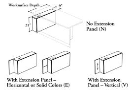
This module supports a Full-Modesty Fixed Run-Off to enable users to work perpendicular to the wall in a sit/stand position. It must be anchored to a building wall.
