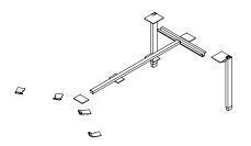
The Dual 120 Angled Worksurface Support bundle mounts to the underside of a worksurface and to the Zig Zag Power Spine Hub to provide support for the worksurface
