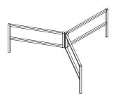
The Power Spine 120 Hub Panel is elevated when finished with required Support Kit.
