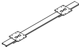
The Centermount Cabinet Support Brackets & Trim provides flush mounted support for centermount cabinets and District overhead cabinets centered on District Panel Walls.
