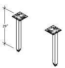
The Height-Adjustable – Leg is used in combination with other legs or storage based supports to create height-adjustable freestanding desks or tables.
