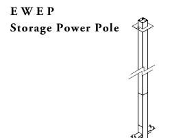
The Storage Power Pole houses the Storage Ceiling Feed and divides the ceiling feed from communication and data cables. It is used to feed power and data to the underside of the storage units.
