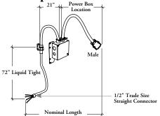
The NYC Split Base Feed connects to the building supply and routes power into the workstation from the wall or floor.
