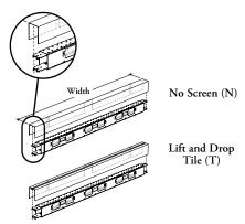
The Chicago EZ Fence Beam for Corridor is a key structural element of the product providing horizontal support for Floor or Modesty Screen – EZ Fence Beam-Mounted. It also carries electricity and data cabling across workstations.
