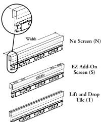
The EZ Fence Beam is a key structural element of the product providing horizontal support for Add-On Screens or a Lift and Drop Tile. It also carries electricity and data cabling across fence.
