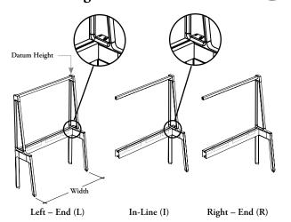
The EZ Fence for Lift and Drop Tile – Single-Sided for Corridor includes all structural components that provide support for all Lift and Drop Tiles and Lift and Drop Vertical Posts It also carries electricity and data cabling across workstations.
