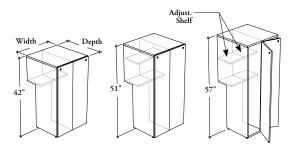
This beam tower provides storage area to store garments and other items for two users, while supporting the front of a worksurface and let a beam pass-through.
