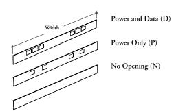
This cover finishes the side of the structural beam.
