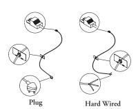
The Input Power Cable brings power from the building ceiling, wall or floor into the Panel Wall.
