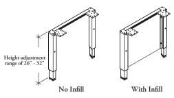
$\label{thm:continuous} The \ Semi-Suspended \ Gable-Height-Adjustable\ provides\ height-adjustable\ support\ for\ worksurfaces\ semi-suspended\ from\ a\ panel\ wall.$
