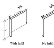
The End Gable provides end of run worksurface support. Available open or with infill options.
