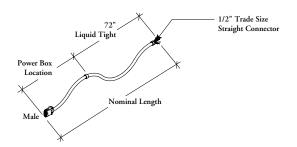
The Base Feed connects to the building supply and routes power into the workstation from the wall or floor.
