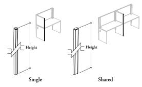
The Lateral Stabilizer – Elements is used to stabilize elements mounted on the side of a desk. It also acts as a finished covering.
