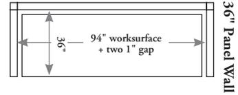
Worksurface is 2" less than the width of the panel wall to allow for a gap on either side.
