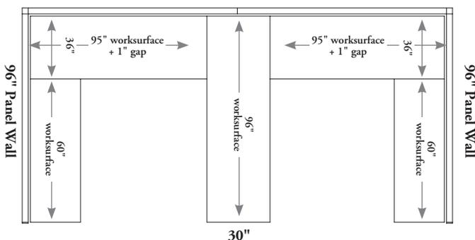
The center worksurface and return remains the full panel width and the outside primary surfaces have a 1" gap.
