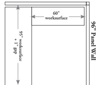
When a semi-suspended worksurface is used, it should be aligned with the panel end. The 1" gap then moves to the corner without having to reduce the return surface by 1".
