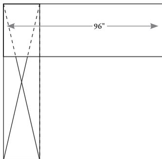
For freestanding applications, gapping is **not** an issue, so a full width worksurface should be specified.
