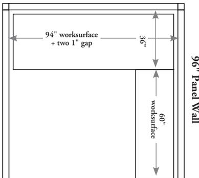
The primary worksurface is wrapped on both sides by panels so it is 2" less than the width of the panel, the return remains the full width.
