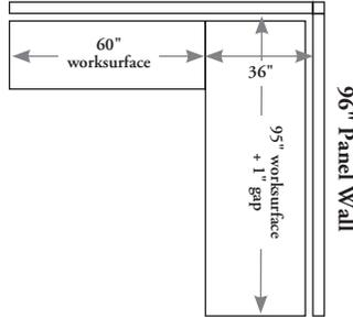
Only the primary surface is 1" less than the width of the panel wall, because there is no gap on the return surface.
