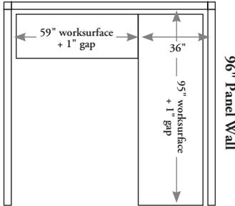
Both worksurfaces are 1" less than the width of the panel walls.
